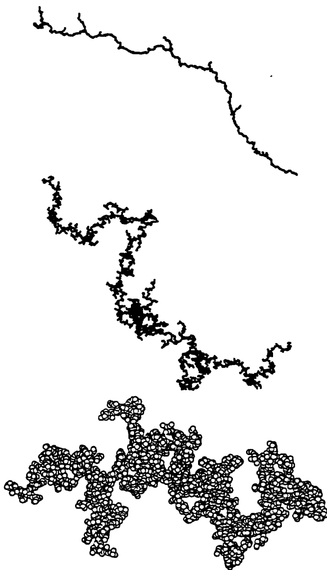
Fig. 2. — Two-dimensional projections of typical three-dimensional aggregates of N = 4096 particles obtained for D = 1.2, 1.6, 2.0 (a) and D = 2.1, 2.3, 2.5 (b).
