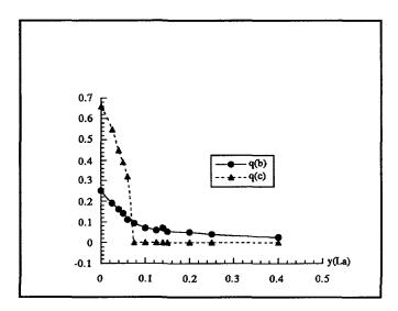
Fig. 4. — Change of  $b^*$  and  $c^*$  wave vector components in Bi<sub>2</sub>(Sr<sub>2-y</sub>La<sub>y</sub>)CuO<sub>6</sub> versus y<sub>La</sub>.
