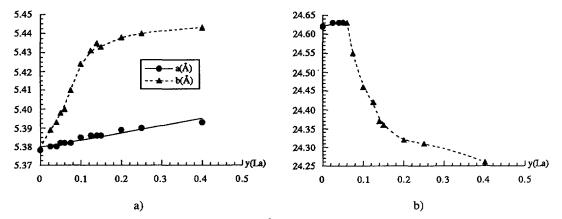
Fig. 5. — Change of lattice constants versus (La<sup>3+</sup>) substitution level, 1) a and b, 2) c.
