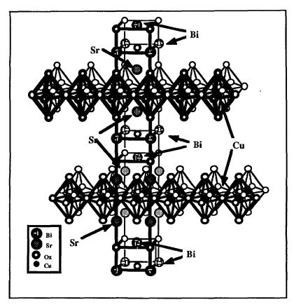
Fig. 1. — Schematic tetragonal structure of Bi<sub>2</sub>Sr<sub>2</sub>CuO<sub>6</sub>.
