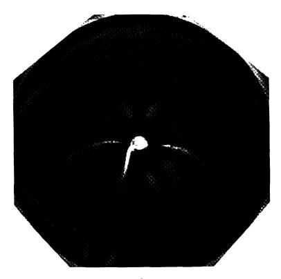
Fig. 2. — Diffraction pattern (MoK<sub> $\alpha$ </sub>) of the 0 kl layer of pure Bi<sub>2</sub>Sr<sub>2</sub>CuO<sub>6</sub>. The modulation wave vector direction is indicated by the Q arrow.
