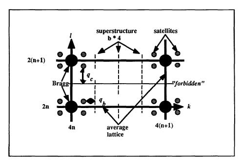
Fig. 3. — Definition of the  $b^*$  and  $c^*$  wave vector components.
