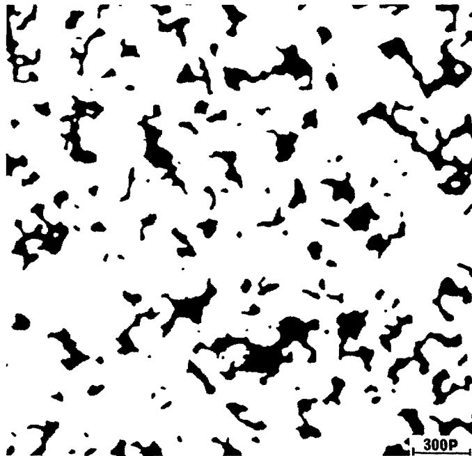
Fig. 1. — Digitized picture of a thin section of dolomite, adapted from reference [27]. The pore network is shown in black. The horizontal bar gives, in pixels, the numerical resolution.
