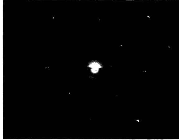
Fig. 4. — [001] zone axis electron diffraction pattern of \text{Bi}_{1.5}\text{Pb}_{0.5}\text{Sr}_2\text{Ca}_2\text{Cu}_3\text{O}_x . Only one set of incommensurate satellites appears which corresponds to a wavevector component along b^* ( \delta' = 0.11 ).
