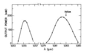
Fig. 3. — Tuning curve of the lamp pumped LNA laser obtained with a lamp excitation power of 2.7 kW. A single-plate birefringent filter with a thickness of 6 mm was used for tuning. The wavelength of the  $2^{3}$ S- $2^{3}$ P transition in helium at 1.083 µm is indicated.
