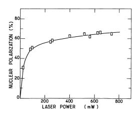
Fig. 5. — Nuclear polarization of a gas of helium-3, obtained in a cell filled with 0.3 torr of gas, as a function of the LNA laser power incident on the cell. The line between the experimental points is just a guide for the eye.
