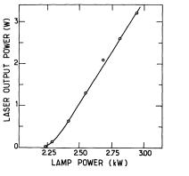
Fig. 2. — Output power of the lamp pumped LNA laser (without selective elements) as a function of the electrical power of the Kr<sup>+</sup> arc lamps. An output coupler with 0.5 % transmission was used. With no selective optics, the laser emitted at 1.08  $\mu$ m and 1.05  $\mu$ m simultaneously.
