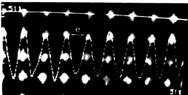
Fig. 4. — Profile corresponding to the center of each row of pores ( $e$  = size of beads).
