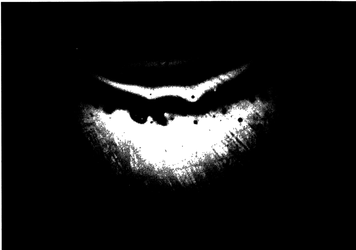
Fig. 1. — Aspect of a drop, as observed through a microscope, by ellipsocontrast techniques. The precursor film appears like a bright halo all around the macroscopic drop. This halo is uniform when the drop is deposited on a bare wafer, but when a silanated wafer is used like in the picture, irregularities of the spreading power of the surface are revealed by the presence of the film, and attributed to inhomogeneities in the grafted monolayer.
