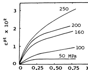
Figure 2 : Variations of deformation due to transformation plasticity versus content of martensite for different applied stresses.
