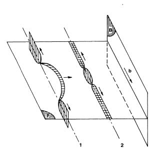
Fig. 3 - Mechanism of glide in a prismatic plane in Beryllium. 1) Unlocking by cross slip from basal to prismatic plane. 2) Locking by cross slip onto the basal plane.
