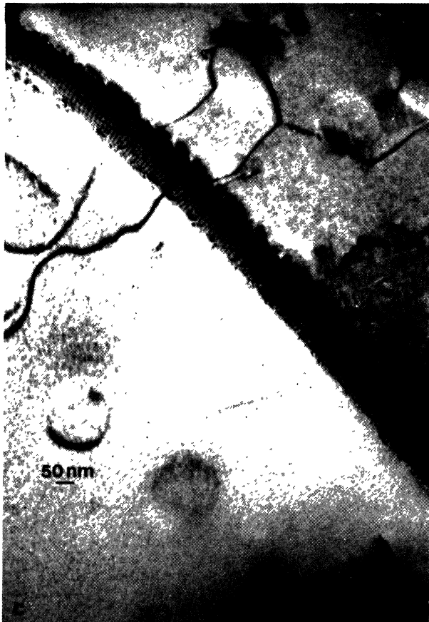
Figure 6. Transmission electron micrographs of dislocation pile ups in Nimonic PE 16 a) shows a planar array crossing a grain b) shows a pile up entering a near \Sigma = 9 boundary and c) shows an individual dislocation entering a low angle grain boundary.
