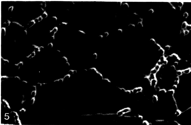
Figure 5 Scanning electron micrograph from sample of type 310 austenitic stainless steel showing variations in the density of M_{23}C_6 precipitates at boundaries. Boundaries with special geometries are marked S whilst those of random character are marked R.
