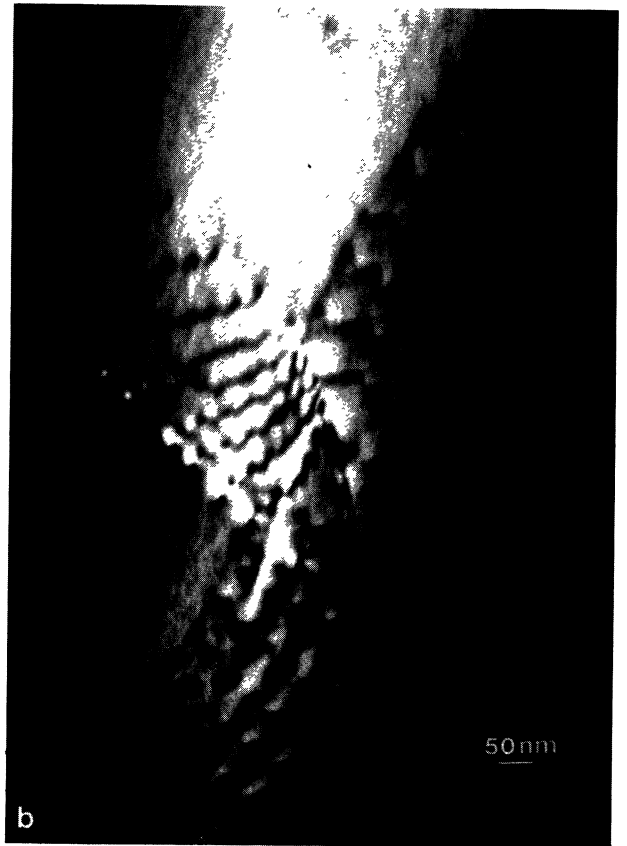
Figure 6. Transmission electron micrographs of dislocation pile ups in Nimonic PE 16 a) shows a planar array crossing a grain b) shows a pile up entering a near \Sigma = 9 boundary and c) shows an individual dislocation entering a low angle grain boundary.
