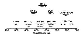
Fig. 1. — Currently available tuning ranges of passively mode locked continuous wave dye lasers. The full names of the saturable absorbers are given in table I.
