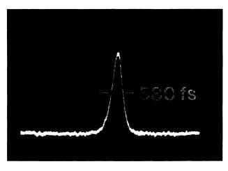
Fig. 4. — Autocorrelation trace of pulses of 580 fs duration obtained at 498 nm using the Coumarin 102 laser mode locked with DOCI.
