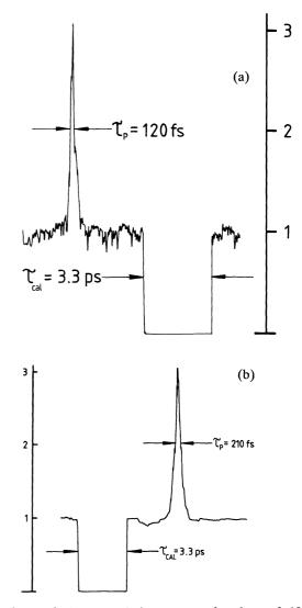
Fig. 3. — a) Autocorrelation trace of pulses of 120 fs duration obtained at 667 nm using the Rhodamine 6G/Sulphurhodamine 101 laser mode locked with DQTCI. b) Typical autocorrelation trace of pulses of 210 fs duration obtained at 561 nm using the Rhodamine 110 laser mode locked with HICI.
