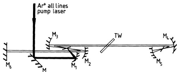
Fig. 2. — Cavity configuration for passively mode locked dye lasers operating from 550 nm to 760 nm.
