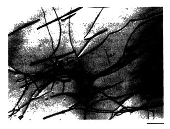
Fig. 5. — Typical dislocation structure observed by TEM in silicon after deformation at the lower yield point at  $T \ge 700$  °C,  $\dot{\gamma} = 2 \times 10^{-5} \text{ s}^{-1}$ ,  $\tau_{\ell_y} \le 10$  MPa, after [32]: bundles of « edge type » dipoles, without precise crystallographic orientations (b, primary Burgers vector, marker: 1 µm).
