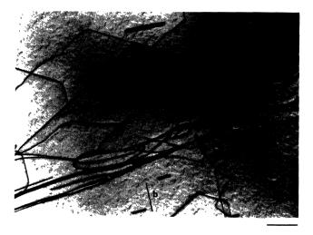
Fig. 8. — Transition between the entangled substructure inherited from high temperature pre-strain and the low temperature substructure (crystallographic orientations) in silicon deformed at T = 550 °C,  $\dot{\gamma} = 2 \times 10^{-5}$  s<sup>-1</sup>,  $\tau = 45$  MPa  $\approx 2/3 \tau_{uy}$ , after [33]. (b, primary Burgers vector, marker : 1 µm).
