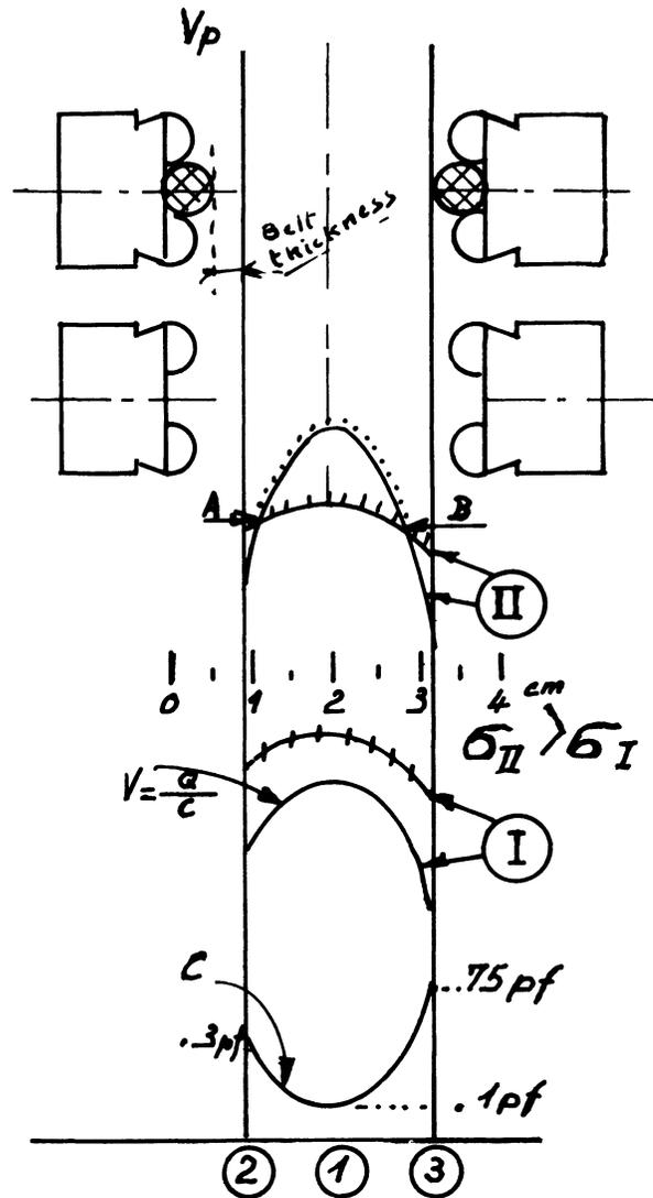
FIG. 8. — Belt voltages compared to Paschen curve in closed structure.
