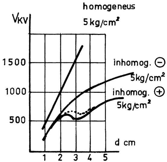
FIG. 3. — Shapes of Paschen curves in SF6 versus distance.
