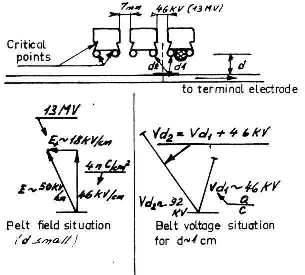
FIG. 5. — Spacers-belt configuration, belt field and belt voltage situation.
