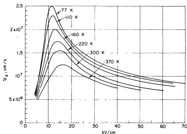
FIG. 30. — Drift velocity vs electric field for electrons in semi-insulating CdTe (Canali *et al.*, Ref. [80]).
