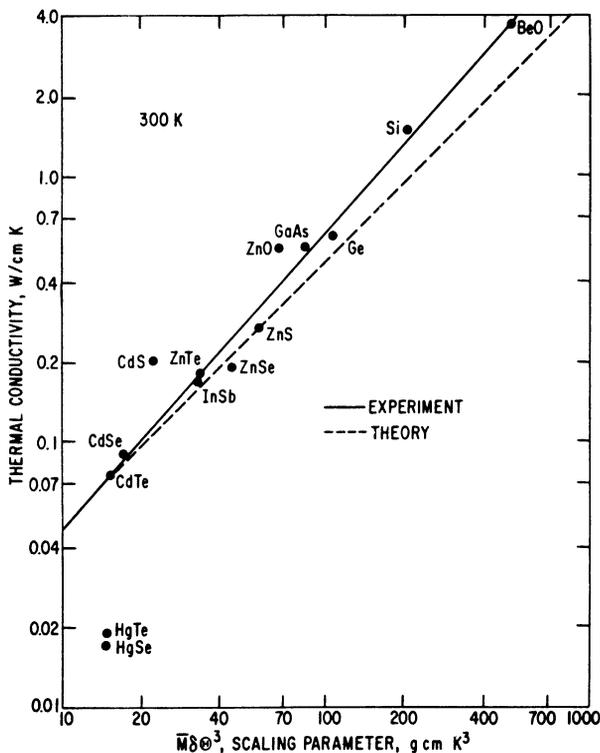
FIG. 9. — Thermal conductivity vs scaling parameter for crystals with tetrahedrally coordinated structures (Slack, Ref. [17]).
