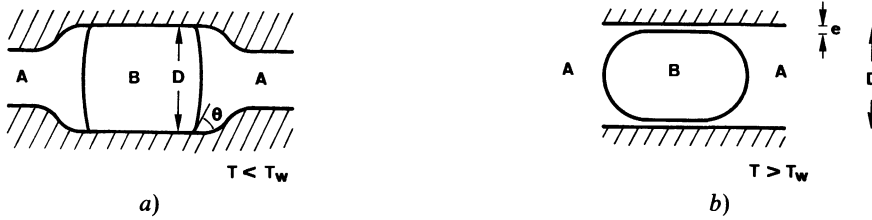
Fig. 2. — A droplet appearing inside one pore : a) partial wetting ; b) complete wetting.
