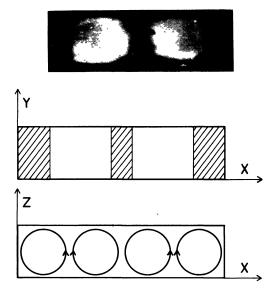
Fig. 1. — Photograph of the cholesteric liquid crystal layer seen from above, and qualitative sketch of the convective rolls. The bright regions correspond to hot ascending fluid, the dark regions to cold descending fluid.
