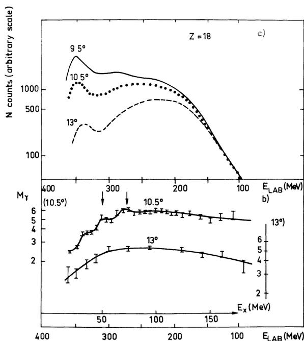
Fig. 1. — Part *a*) Kinetic energy spectra (lab.) of the  $Z = 18$  fragment at  $9.5^\circ$ ,  $10.5^\circ$ ,  $13^\circ$ . The relative scaling of the number of counts is arbitrary. Part *b*) Multiplicity spectra at  $10.5^\circ$  and  $13^\circ$  (lab.). The arrows show the position of the structures observed in ref. [3] in  $^{37}\text{Ar}$  isotopes. Only statistical uncertainties are indicated. The total excitation energy is also indicated.
