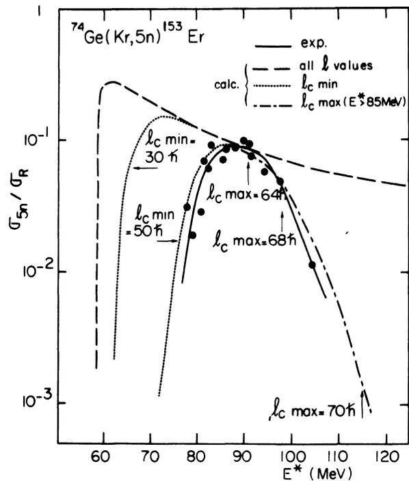
FIG. 3. — Excitation function for the reaction  $^{74}\text{Ge}(\text{Kr}, 5n)^{153}\text{Er}$ . Same caption as in figure 2. Attempts for different  $l_c$  values are shown on the low side and high side :
