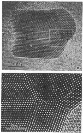
In an analogous manner to  $<100>_{A1}$  needles,  $<110>_{A1}$  needles also display multiply-twinned morphology. Figure 5 is an example of such a precipitate. In the enlargement in fig.5 (b), the convergence of the five twin segments is clearly visible.
