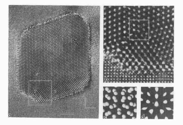
Fig. 3 : Bright field micrograph showing the morphology of Ge precipitate in a bulk-aged sample. Note the alignment along the <100> direction in Al (for the simulation (d), defocus = -80 nm, thickness = 5 nm).
