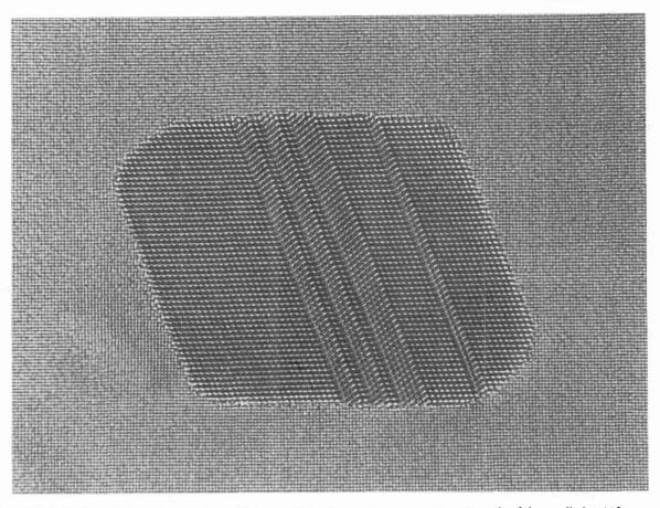
Fig. 2 : High resolution micrograph in which a needle is observed in cross-section. The axis of the needle is  $<110>_{Ge}$  parallel to a  $<100>_{AI}$  direction. No relaxation into a dislocation structure is apparent at either type of interface.
