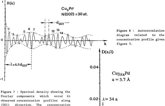
signal has been smoothed over 10 a (a is the lattice parameter) in such a way to enhance low range frequencies
