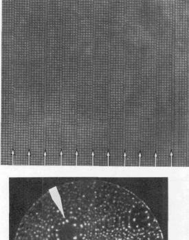
Figure 2 : High resolution image of the LPS M = 6.24 observed in Cu - 20.5 Pd at 485°C. White dots represent Pd columns. Arrows indicate the mean positions of the APB's which are spread over two planes.
