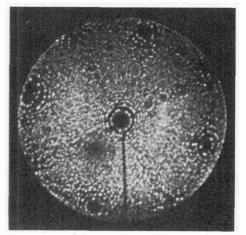
Figure 4 : Field ion image of Cu 18.5%Pd. The absence of discontinuities on the central (001) pole indicates that APB's are perpendicular to the tip axis (analysis direction). The tip radius is here close to 800 Å.
