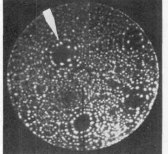
Figure 3 : Field ion image of Cu 18.5 % Pd. The tip radius is close to 400 Å and the average magnification is around 1.6  $10^6$ . The array of parallel APB's leads to well visible discontinuities at the vicinity of the central (001) pole.
