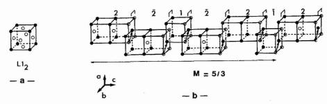
Figure 1 : a) The  $Ll_2$  structure consists in a stacking of alternate pure A planes and mixed AB planes. b) Long Period Structure such as M = 5/3; the APB's are lying in (001) planes, the antiphase vectors indicated by arrows, belong to the plane of antiphase. Only atoms in the mixed planes (001) are shown. The structure is such that three APB are displayed over five  $Ll_2$  cubes according to the sequence 221.
