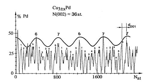
Figure 5 : This concentration profile shows the stacking sequence of (002) planes in Cu 20.5 at % Pd and the long range modulations associated to conservative APB's ( $\perp$  (001)).
