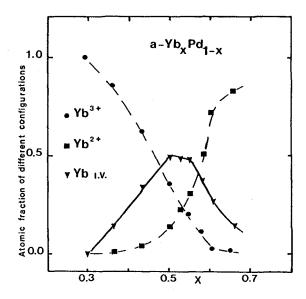
Fig. 3. – Fractions of the different charge states versus composition in the amorphous Yb-Pd alloys.
