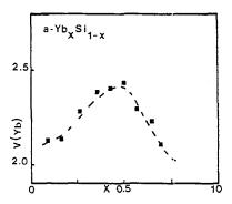
Fig. 4. - Mean valence in the amorphous Yb-Si alloys.
