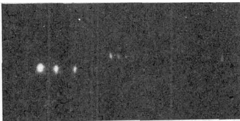
Figure 7a (above). Imaging test at 44.7 Å with Spherical Off-Axis Imager Telescope in the MSFC 1000 ft vacuum chamber. Exposures are 3 hr, 1 hr, 20 min, 10 min, 4 min, 2 min, 1 min, and 30 seconds in duration. The five shortest exposures are separated by 10 arcseconds each. Plate scale on the film is 3 microns/arcsecond.
