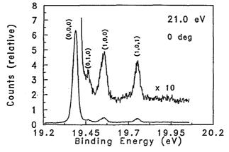
Figure 1: Photoelectron spectrum of the  $\tilde{C}$  state of  $CO_2^+$  taken at 21.0 eV photon energy,  $\theta=0^\circ$ , and 2 V pass energy.
