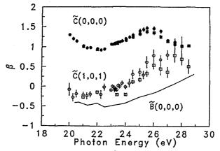
Figure 2:  $\beta$  results for the  $\tilde{C}(0,0,0)$  and  $\tilde{C}(1,0,1)$  vibrational levels of  $C0_2^+$ . Results for 2 V (squares) and 5 V (circles) pass energy are shown. Experimental results of Grimm et al. [5] for the  $\tilde{B}(0,0,0)$  state as a function of <u>kinetic</u> energy are connected by the solid curve.
