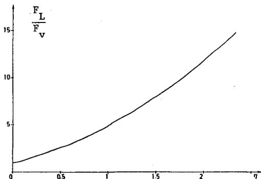
Figure 3 - The ratio of the linear fraction  $F_L$  to the actual volume fraction versus the analysis parameter  $\eta$
