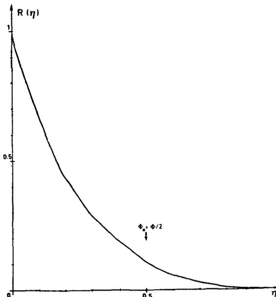
Figure 4 - The ratio of resolved particles as a function of the analysis parameter  $\eta$ .
