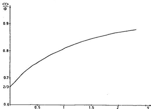
Figure 2 - The ratio of the mean apparent length  $\langle l \rangle$  to the precipitate diameter  $\phi$  as a function of the analysis parameter  $\eta = \phi_a / \phi$ .
