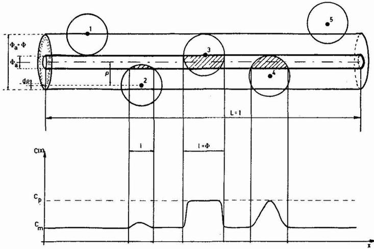
Figure 1 - Atom-probe analysis of a decomposed alloy. The particles are respectively being not detected (1), detected but not resolved (2), clearly resolved (3), close to be resolved (4), not detectable (5)
