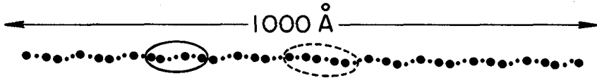
Fig.5. The dislocation structure as seen in electron microscopy[2,8] of a \theta=[\bar{2}09] tilt boundary in NiO. Note the two different spot sizes, which is indicative of Burgers vectors of two different lengths. The dashed line encloses a defect in the faceting structure of the boundary.
