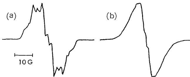
Fig. 2 - Effect of anisotropic term of hyperfine coupling on simulated ESR spectra of randomly oriented immobile solitons. Curve (a) is the result for the isotropic coupling only. Curve (b) is that including anisotropy. Anisotropic term tends to wash out the structure of the curve (a). Parameter values for A and \alpha are 30 gauss and 0.5 respectively. Natural width of 0.8 gauss is assumed.
