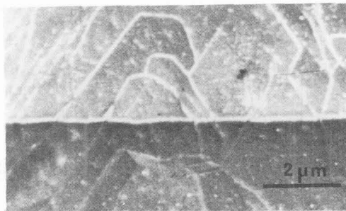
Fig.3b): SEM secondary electron image of the same p-n junction region after Schimmel etch
