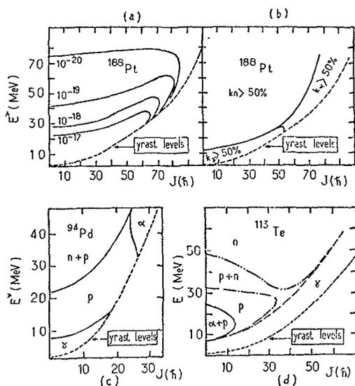
Fig. 17 - Contour plots in the plane  $E^*$  versus  $J\hbar$ , for the compound nuclei  $^{188}\text{Pt}$ ,  $^{94}\text{Pd}$  and  $^{113}\text{Te}$ , according to calculations made by Delagrangé et al [53]: a) Life time, b), c) and d) probabilities higher than 0.5 for emission of neutrons, protons,  $\alpha$  particles and  $\gamma$  radiation.
