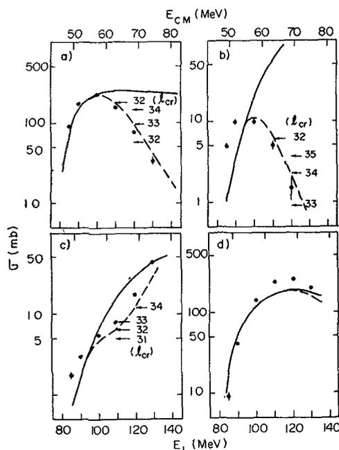
Fig. 18 - Determinations of  $l_{\text{cr}}$  values on the systems  $^{34}\text{S}+^{45}\text{Sc}$  by Langevin et al [48]. Excitation functions correspond to the following excitation channels: a)  $2pn$  and  $2np$ , b)  $2p,np$  and  $2n$ , c)  $\alpha n$  and  $2p3n$ , d)  $3np$ ,  $2p2n$  and  $3pn$ . The lines correspond to the code ALICE (solid lines - all partial waves, dashed lines - indicated  $l_{\text{cr}}$  values).
