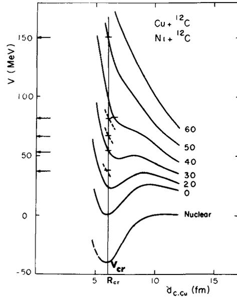
Fig. 10 - Calculated potential energy curves for the system  $(Ni + {}^{12}C)$  at various  $\ell$ h values (ref. [33]). Experimental critical  $\ell$  values were obtained at various energies by Namboodiri et al [41]. The critical potential is shown, close to the bottom of the nuclear potential, at  $R_{cr} = (Z_1 Z_2 / A_1^{1/3} + A_2^{1/3})$ , i.e. for  $r_{cr} = 1$  fm.
