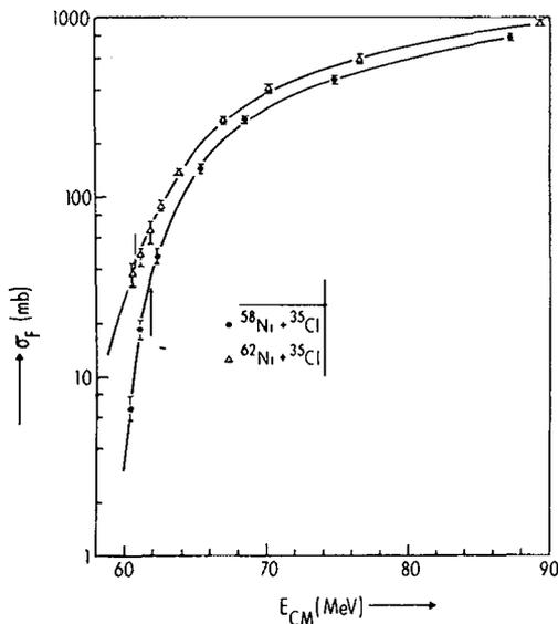
Fig. 3 - Excitation functions for complete fusion (evaporation residue) cross sections for  $^{35}\text{Cl}$  induced reactions on two nickel isotopes (After Scobel et al [16])
