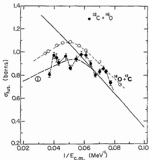
Fig. 7 - a) Excitation function for complete fusion in the systems ( $^{18}\text{O} + ^{12}\text{C}$ ) (After ref. 27). At low energies,  $\sigma_{\text{CF}}$  versus  $1/E$  follows a straight line as predicted by equation (5). At higher energies the critical distance for complete fusion rules the cross section calculation according equation (13), with  $V_{\text{cr}} = -14$  MeV and  $r_{\text{cr}} = 1.01$  fm.
