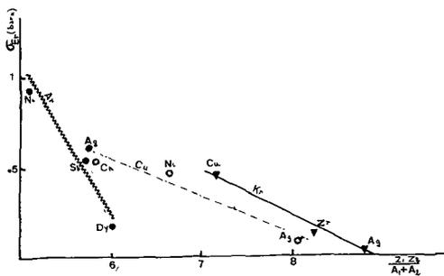
Fig. 19 - Cross section for evaporation residues as a function of the parameter  $Z_1Z_2/(A_1+A_2)$  in argon induced reactions on Ni, Sb, Ag and Dy [45], copper induced reactions on Ni and Ag, chromium on iron [54], and krypton on Cu, Zr and Ag [55].
