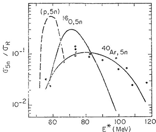
Fig. 15 - Excitation functions for 5 neutrons emitted by a compound nucleus  $^{150}\text{Er}$  produced by proton,  $^{16}\text{O}$  and  $^{40}\text{Ar}$  projectiles. Experimental points are shown for the ( $^{40}\text{Ar},5n$ ) reaction.
