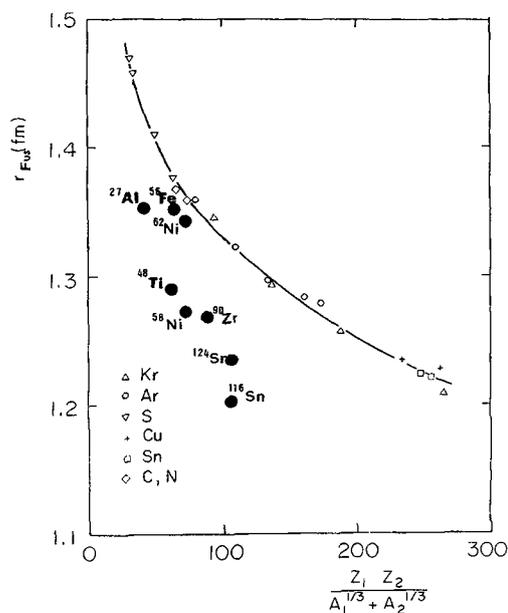
Fig. 6 - Plot of  $r_{\text{Fus}}$  (calculated by Ngô et al [22], versus  $Z_1 Z_2 / (A_1^{1/3} + A_2^{1/3})$ ). The full curve represents the average behavior. Dark points are deduced from Scobel et al.'s experimental cross sections [16].
