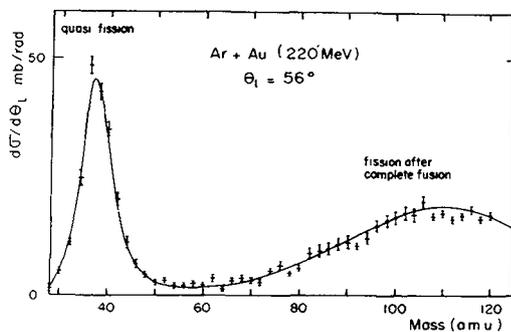
Fig. 21 - Mass distribution for the fragments produced in the reaction  $^{40}\text{Ar} + ^{197}\text{Au}$  at 220 MeV. There is a very clear distinction between quasi-fission or deep inelastic light fragments around  $A = 40$ , and fission fragments [63].
