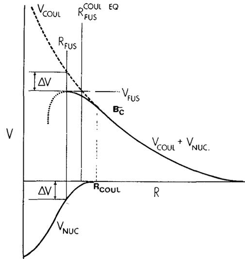
Fig. 4 - Potential energy versus distance, R, between two complex nuclei. Complete fusion occurs only when  $V_{\text{FUS}}$  is overcome.  $\Delta V$  is the nuclear potential at the distance  $R_{\text{FUS}}$  where  $dV/dR = 0$ .  $R_{\text{FUS}}^{\text{Coul.Eq}}$  is the equivalent radius obtained applying a pure Coulomb repulsion.
