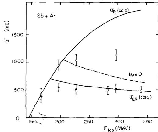
Fig. 20 - Cross sections for evaporation residues in the reaction ( $^{40}\text{Ar}+\text{Sb}$ ). Dark points : experimental results [45]. Open circles :  $\sigma_{CF} = \sigma_{ER} + \sigma_{fiss}$ .  $\sigma_{ER}$  calculated has been obtained with the ALICE code. The dashed curve with  $B_f = 0$  is the calculated  $\sigma_{CF}$  using the rotating liquid drop fission barrier as a limit for  $\ell_{cr}$ .
