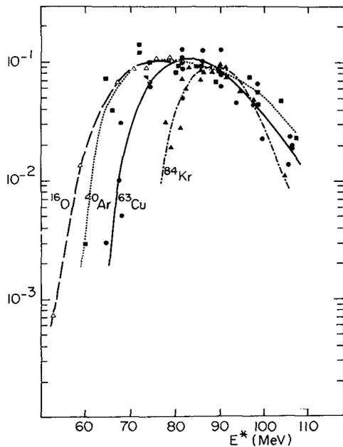
Fig. 22 - Excitation functions for (HI,5n) reactions passing through the same compound nucleus  $^{158}\text{Er}$  ( $^{159}\text{Tm}$  for  $^{63}\text{Cu}$  projectiles). The shift between  $^{16}\text{O}$  and  $^{84}\text{Kr}$  is clearly seen [75-76].
