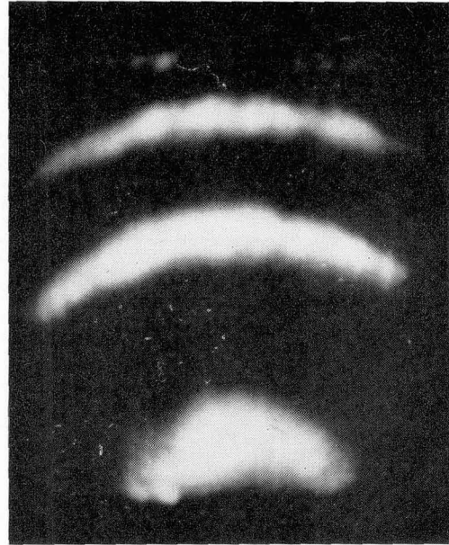
FIG. 1. — Interferogram recorded by channelled image intensifier. Spectral resolving power 10^4 .
