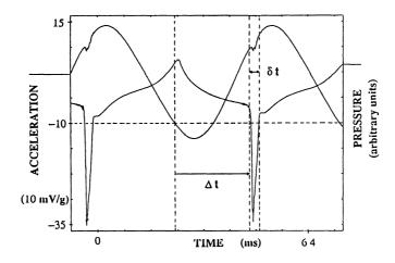
Fig. 2.— Acceleration and pressure as functions of time. The grain layer loses contact with the vessel base when the acceleration is less than -g. The sharp peaks of the pressure signal indicate the collisions with the vessel base. We can thus measure the flight time, the collision time and the collision duration.
