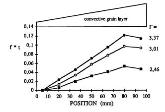
Fig. 4.— Collision time *t versus* position, measured with the seven transducers, for three acceleration values, and a schema of the shape of the heap  $(f = 20 \text{ Hz}, N \approx 45)$ . One observes the propagation with a constant speed of the collision front, from the thinner to the thicker part of the convective heap. The collision time difference increases linearly with  $\Gamma$ .
