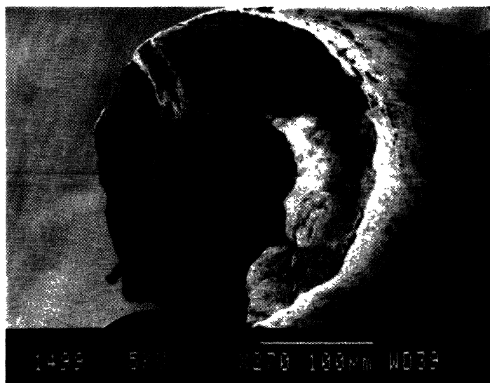
Fig. 1.— Scanning electron microscope photographs of melt-spun copper laurate fibres. Anisotropic contraction upon cooling is indicated by the corrugated surface (a) and the central hole (b). A microfibrillar structure is seen on the fracture surface (a).
