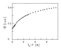
Fig. 5. — The temperature dependence of the tilt angle of the molecules in the  $SmC^*$  phase.
