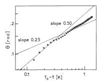
Fig. 7. — The temperature dependence of the tilt angle  $\theta$  near  $T_{\rm c}$ .
