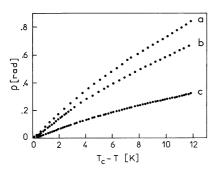
Fig. 2. — The measured rotatory power as a function of temperature for three different wavelengths; (a) for  $\lambda_1 = 488 \text{ nm}$ ; (b) for  $\lambda_2 = 515 \text{ nm}$  and (c) for  $\lambda_3 = 647 \text{ nm}$ .
