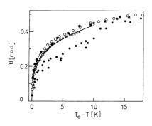
Fig. 6. — Measurements of  $\theta(T)$  obtained by unwinding of the helix; (•) data from reference [10], (\*) data from reference [8] and (O) data from reference [13]. Our results obtained in an unperturbed helix structure : (x). The solid line is a fit to our results of the form  $(T_c - T)^{\beta}$ .
