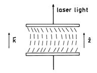
Fig. 1. — The geometry of the sample in the rotatory power experiment. The wave vector of the helical structure is perpendicular to the wall surfaces.
