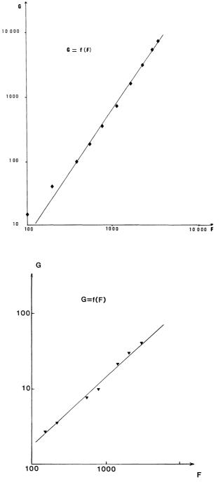
Fig. 2. — Log-log plot of the conductivity (in arbitrary units) as a function of the macroscopic force (in Newtons), a) for a disordered packing of spheres (h = 41 mm, 35 000 spheres), b) for an ordered packing of 1 600 cylinders; the fluctuations at high pressure become very important.
