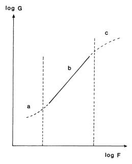
Fig. 1. — Schematical behaviour of conductivity vs. the pressure in log-log scale and arbitrary units : a) consolidation phase, b) experimental region, c) asymptotic behaviour (not reached practically).
