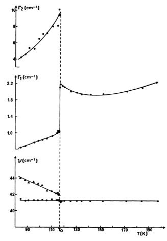
Fig. 4. — Linewidth and frequency temperature dependence at  $P = 3\,000$  bar of the two lowest frequency modes of hydrogenated p-terphenyl. On the  $\nu = f(T)$  diagram, points correspond to mode 1 whereas triangles are relative to mode 2.
