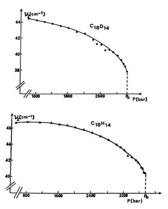
Fig. 8. — Linewidth pressure dependence of the « softening » mode of deuterated and hydrogenated p-terphenyl.
