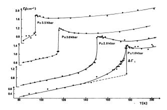
Fig. 6. — Linewidth temperature dependence at four different pressures of the lowest frequency mode of hydrogenated p-terphenyl.
