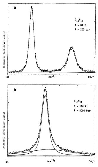
Fig. 2. — Refinements of experimental spectra exhibiting two modes by two Lorentzian functions. These examples of refinements are presented for two limit cases : (a) the two modes are well separated, (b) the two modes overlap. Circles correspond to experimental points and the different curves are the results of refinements.
