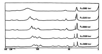
Fig. 1. — Evolution of the low frequency spectrum of the hydrogenated p-terphenyl at different pressures and at constant temperature T = 84 K. ( $P_0 = 3750$  bar). The arrows indicate the soft mode.
