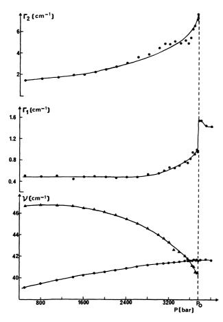
Fig. 3. — Linewidth and frequency pressure dependence at T = 84 K of the two lowest frequency modes of hydrogenated p-terphenyl. On the  $\nu = f(P)$  diagram points correspond to mode 1 whereas triangles are relative to mode 2.
