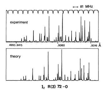
Fig. 2. — Hyperfine structure of the R (3) 72-0 B  $\leftarrow$  X transition. The wavelength scale is given by the lambdameter. It is calculated from a third order polynomial fit to the lambdameter measurements obtained during the laser frequency scanning. The relative precision is of the order of 1 MHz. The upper trace is the transmission fringes of a confocal Fabry-Perot of 81 MHz F.S.R., used as a monitor of the laser scan. The R.M.S. deviation in the fit to the recorded spectrum is 2.5 MHz.
