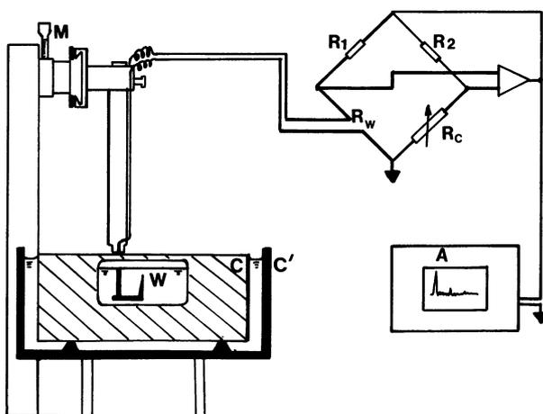
Fig. 1. — Experimental set-up.  $W$  : hot-wire;  $C$  : tank;  $C'$  : thermostatic bath;  $M$  : micrometric pedestal;  $A$  : spectrum analyser;  $R_1, R_2, R_3, R_4$  : Wheatstone bridge, constant temperature anemometer.
