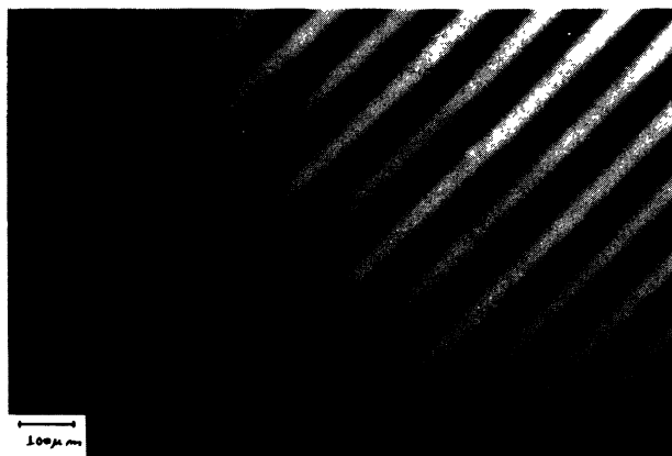
Fig. 7. — Calamitic SdS ferrocholesteric in a microslide 200 \mu\text{m} thick a few hours after removal of the magnetic field (applied along the X direction). Crossed polarizers, observation along the z direction. Hydrodynamic instabilities, roll structure.
