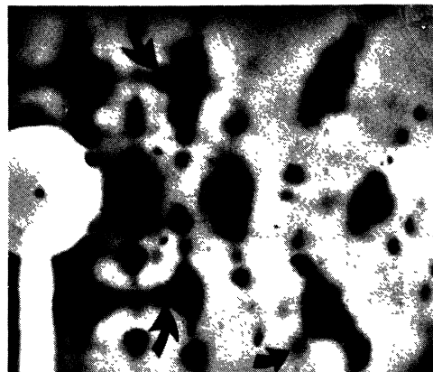
Fig. 7. — X-ray pattern of (\text{TMTSF})_2\text{BrO}_4 at 11.5 K showing midway between layers of main Bragg reflections broad superlattice spots (arrow). Note very strong diffuse scattering surrounding main Bragg reflections. On this pattern the a direction is horizontal.
