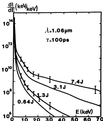
Fig. 6. — Typical X-ray spectra obtained at  $\lambda = 1.06 \mu\text{m}$ ;  $\tau = 100$  ps and fluxes of  $1.3 \times 10^{14}$ ,  $2.6 \times 10^{14}$ ,  $6.3 \times 10^{14}$  and  $1.5 \times 10^{15}$  W/cm<sup>2</sup>.
