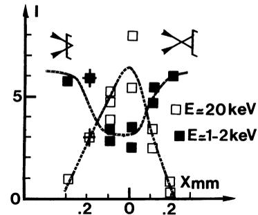
Fig. 1. — Soft (1-2 keV) and hard (20 keV) signal *versus* target position.  $\lambda = 1.06 \mu\text{m}$ ;  $\tau = 100$  ps. The dotted lines follow the mean values of the data. Crosses are the error bars for each shot.
