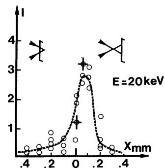
Fig. 2. — Hard X-ray signal (20 keV) *versus* target position.  $\lambda = 1.06 \mu\text{m}$ ;  $\tau = 2.5$  ns. The dotted line follows the mean values of the data. Crosses are the error bars for each shot.
