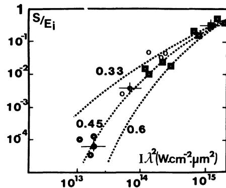
Fig. 8. — Hard X-ray signals  $S(E \approx 15$  keV) normalized to incident energy  $E_i$  versus  $I\lambda^2$ . Different theoretical curves are for  $T_H = a(I\lambda^2)^\alpha$  for different  $\alpha$ .
