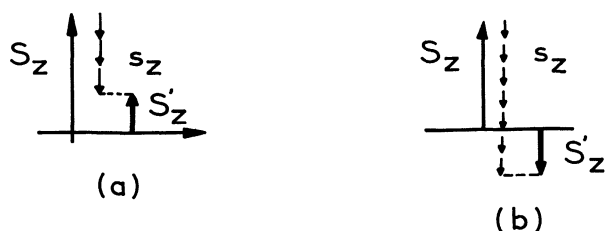
Fig. 2. — The strong coupling arrangement of spins for the impurity and n trapped electrons (a) when n < 2S , (b) when n > 2S .
