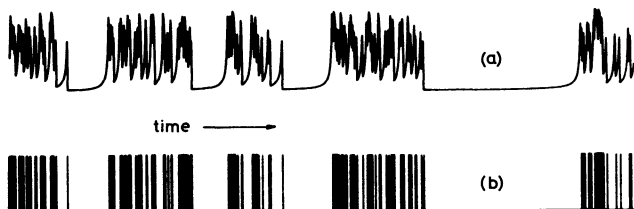
Fig. 1. — a) Example of intermittent signal obtained from the model defined by equation (1). b) Forgetting the underlying dynamics, one can consider this signal as a succession of noises whose distribution is of interest.
