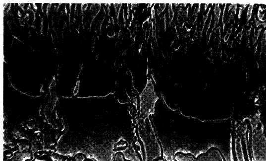
FIG. 1. — A 3 % solution of cholesteryl oleate in methoxybenzylidene-butylaniline observed between crossed polarizers with white light. The sample is flowing and many singular lines can be seen.
