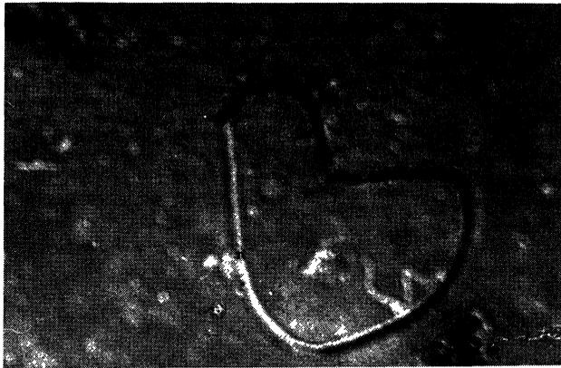
FIG. 14. — Quasi-static *wall* appearing at the meeting zone of dislocations travelling in opposite directions. These dislocations had just wiped off the structure deformations produced by the dilative stress. Under stresses this wall is able to emit the thin light lines which are suggested to be small burgers vector dislocations (see text).
