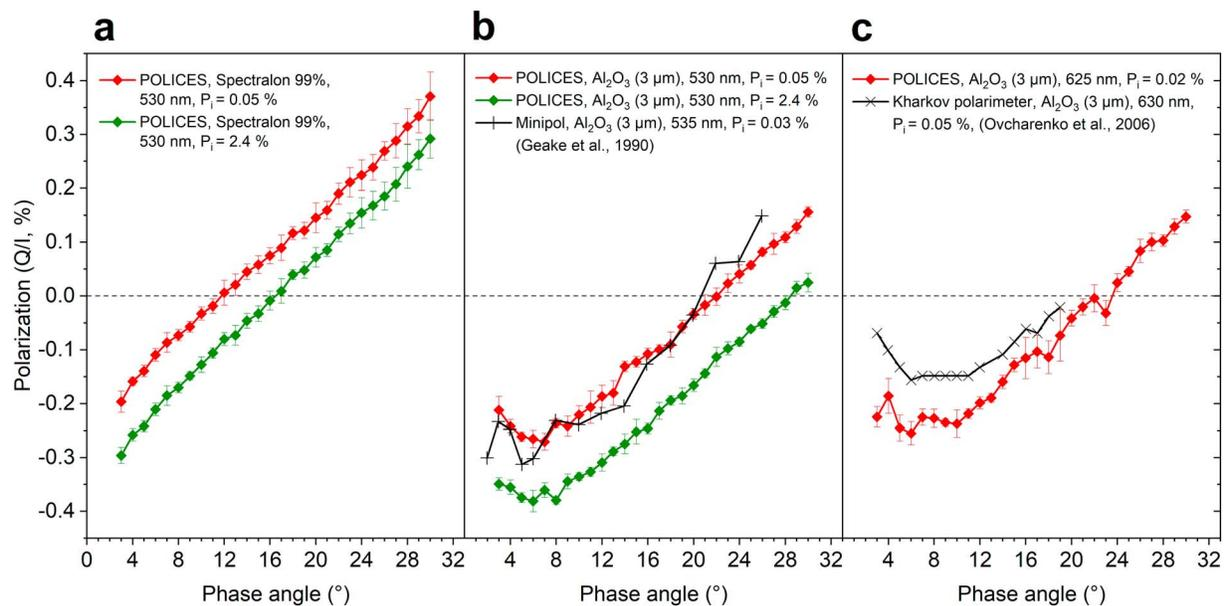
**Figure 2.** Measurements of (a) Spectralon with and without depolarizer, (b) surface made of 3- $\mu\text{m}$ -diameter aluminum oxide (WCA3) with and without depolarizer and as measured by Geake and Geake (1990), and (c) same surface measured with depolarizer at 625 nm compared to measurement by Ovcharenko et al. (2006) at 630 nm. The red phase curves are available in Data Set S1. POLICES = POLarimeter for ICE Samples.
