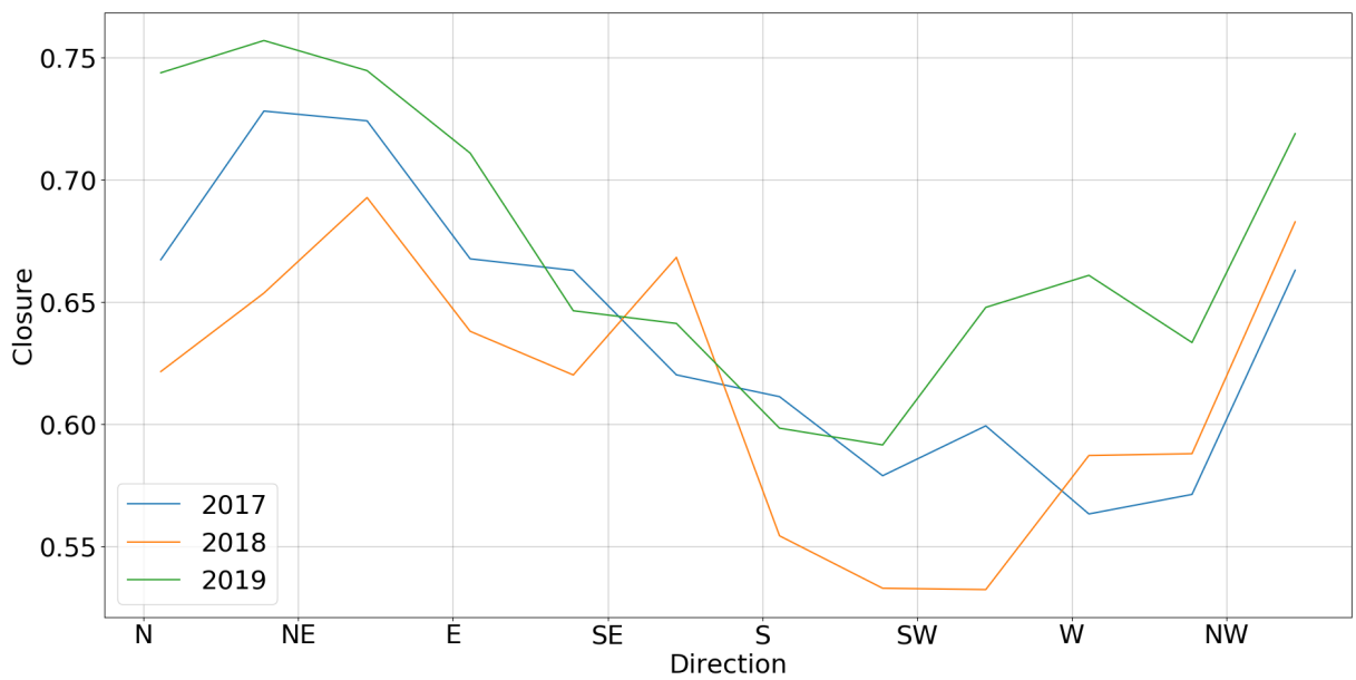
Fig. A4: Dependence of the energy budget closure on the wind direction for all three summers.
