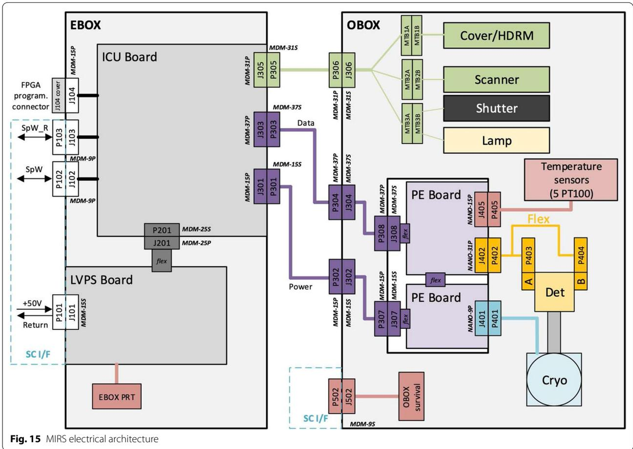
Fig. 15 MIRS electrical architecture
