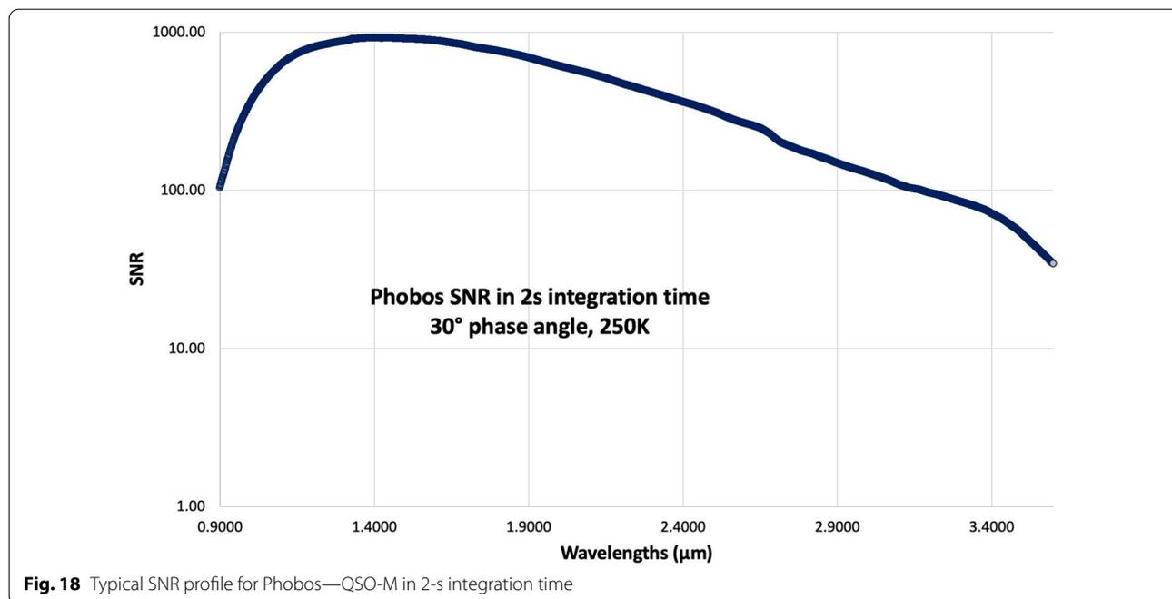
**Fig. 18** Typical SNR profile for Phobos—QSO-M in 2-s integration time
