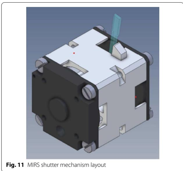
Fig. 11 MIRS shutter mechanism layout
