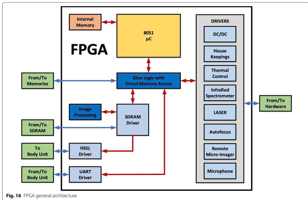
Fig. 16 FPGA general architecture
