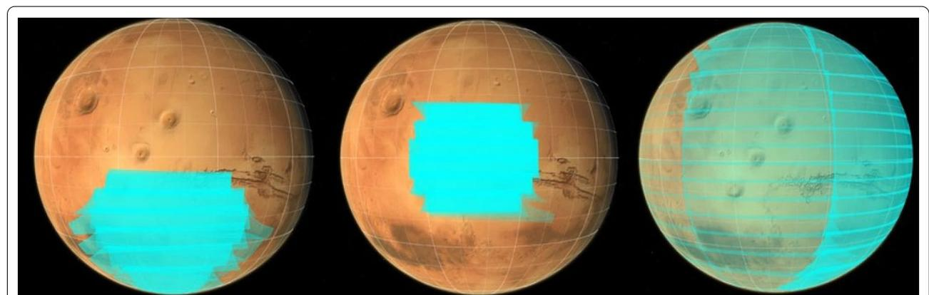
**Fig. 21** Example of Mars observations on QSO-M Dec 2027. Left: 3 observations of South hemisphere with 45 min time resolution: 1h30 time span. Center: 5 observations of a central zone with 30-min time resolution: 2 h time span. Right: global coverage of lighted part of Mars
