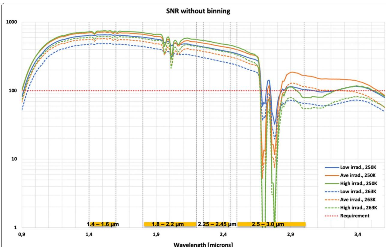
**Fig. 19** Mars SNR in different radiance cases. SP#1: simulated MIRS SNR for the average Mars radiance observed by VIRTIS during Rosetta flyby (Coradini et al. 2010). SP#2: SNR for simulated Mars radiance at Ls 150° over dark highlands. SP#3: SNR for simulated Mars radiance at Ls 270° over Hellas Basin. SP#4: SNR for simulated Mars radiance at Ls 60° over the north plains
