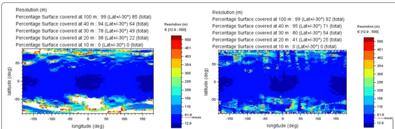
**Fig. 20** Left: example of geometric resolution for equatorial QSO-M Nov 2025 ( $\beta = 3^\circ$ ). Most of Phobos is covered with high resolution. Zones in white cannot be observed because of MMX equatorial trajectory and Phobos flat shape on highest latitudes (poles). Right: example of geometric resolution for 3D-QSO-M Sep–Oct 2026 ( $\beta = -6^\circ$ ). Highest latitudes (poles) can be observed thanks to MMX 3D trajectory that allows visibility of high latitudes
