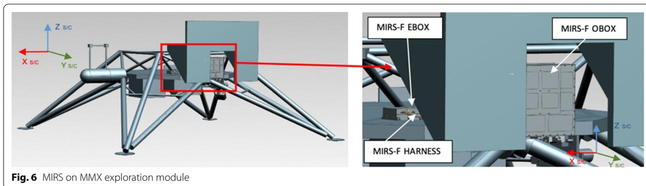
**Fig. 6** MIRS on MMX exploration module
