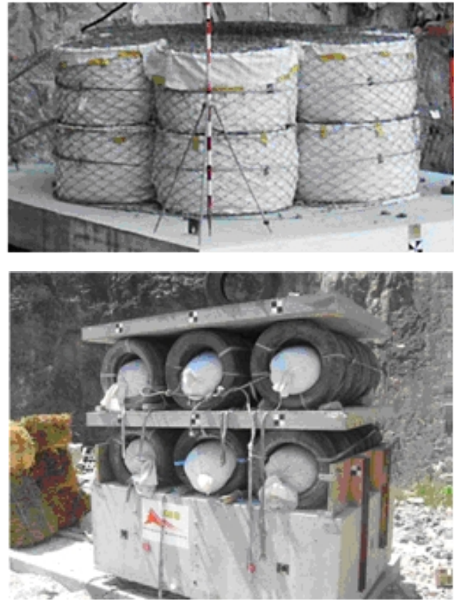
Fig. 14. Alternative cushion layers: (top) Fence box structure with cellular glass material (Schellenberg, 2008), (bottom) Multi-layer sandwich structure (Lorentz et al., 2008).
