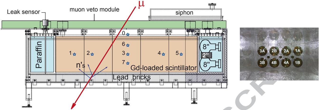
Figure 3: *Left*: general layout of the neutron counter detector, positions of LED's are indicated by stars. *Right*: a view from inside of the installed but not yet filled scintillator chamber, 8 of the 8-inch and 3 of the 2-inch PMTs are seen. Numbers indicate different PMT groups consisting of two 8-inch PMTs (A,B) each.
