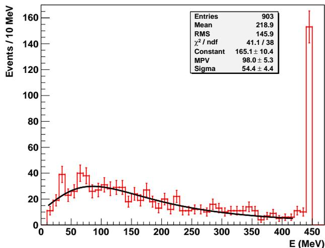
Figure 6: Energy deposition measured with the *muon PMT's* of NC for the events in coincidence with the  $\mu$ Veto module on top of the NC, live time is 177.9 days. Last bin contains events with energy deposition of  $E \geq 440$  MeV (overflow bin). Landau distribution is fitted to the data and calibrated with MC simulations of muons passing through the NC.
