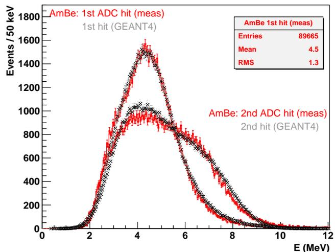
Figure 7: Energy spectra acquired with AmBe source (spectra of the first and second ADC hits are shown) (*solid lines*). Both ADC hits of AmBe measurement are compared with corresponding GEANT4 simulations (*crosses, dashed line*)(see text for details).
