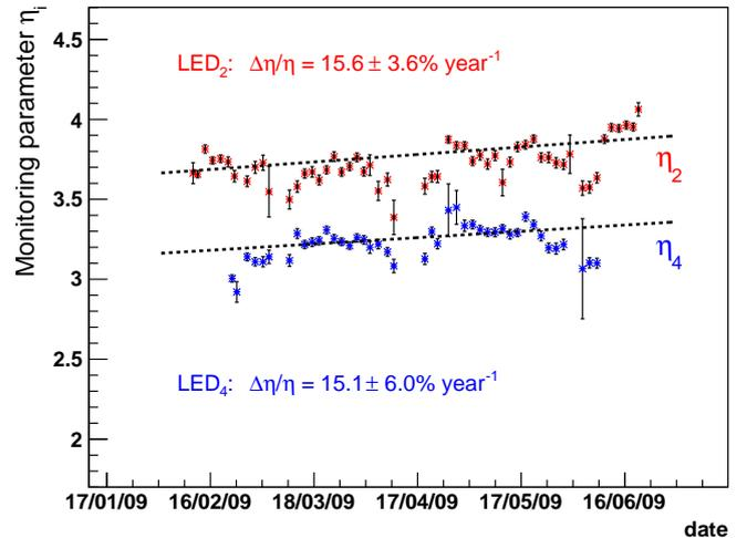
Figure 5: Long term behaviour of the scintillator transparency: 4-months trends of the  $\eta$  ratio for two non-central LED's: LED<sub>2</sub>(top) and LED<sub>4</sub>(bottom) (see Sect. 4.1 for details). Both data sets are fit independently with a linear function.
