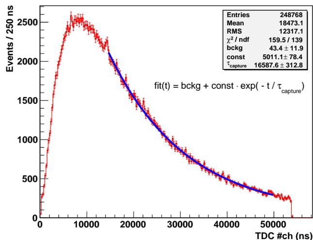
Figure 8: AmBe measurement: time difference between a start of the event (first hit) and any following TDC hit within the acquisition time. The falling edge is fit with an exponential function and a flat background component.
