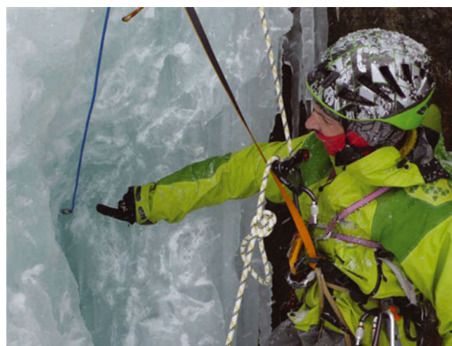
Fig. 3. Extraction of the pressure sensor from the ice of the Nuit Blanche free standing at the end of the season (picture taken on 13 March 2008). The sensor was embedded inside \sim 60 cm of ice
